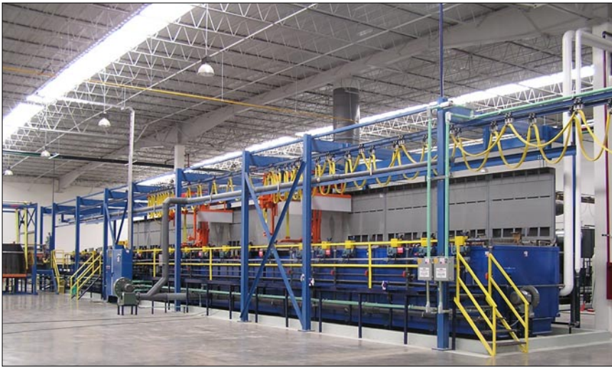
Double row push-pull ventilation
